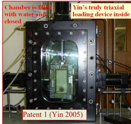
(b) The patent of "truly triaxial loading device:" in Yin (2005) has been used by Tsinghua University (Top 14 in QS World University Rankings 2023). Results from the true trial tests were used of design & construction of a large "Rumei Core Wall Rockfill Dam of 315 m high with total investment of RMB60 billion (C\$12 billion). Please see a letter dated 6 May 2022 from Tsinghua University.
